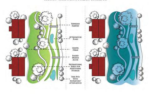
Figure 38. Concept plan of stream corridor and flood storage area (Utilis 2018)
