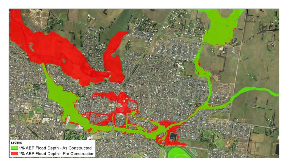
Figure 13. Flood extent reductions due to flood mitigation works (Water Technology 2017)
