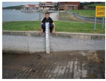
Figure 26. Simpson Street boat ramp water level monitoring board
