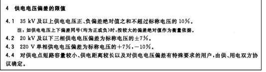
Figure 3.11: In GB/T 12325-2008 on Voltage Deviation Limit
