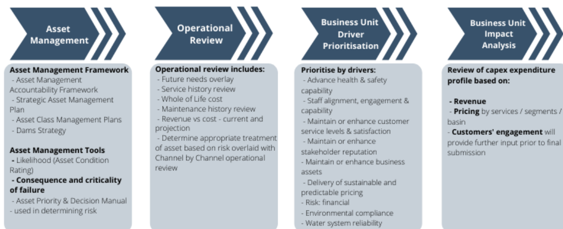
Figure 2: Process for Risk Determination, Project and Program Capex Development
