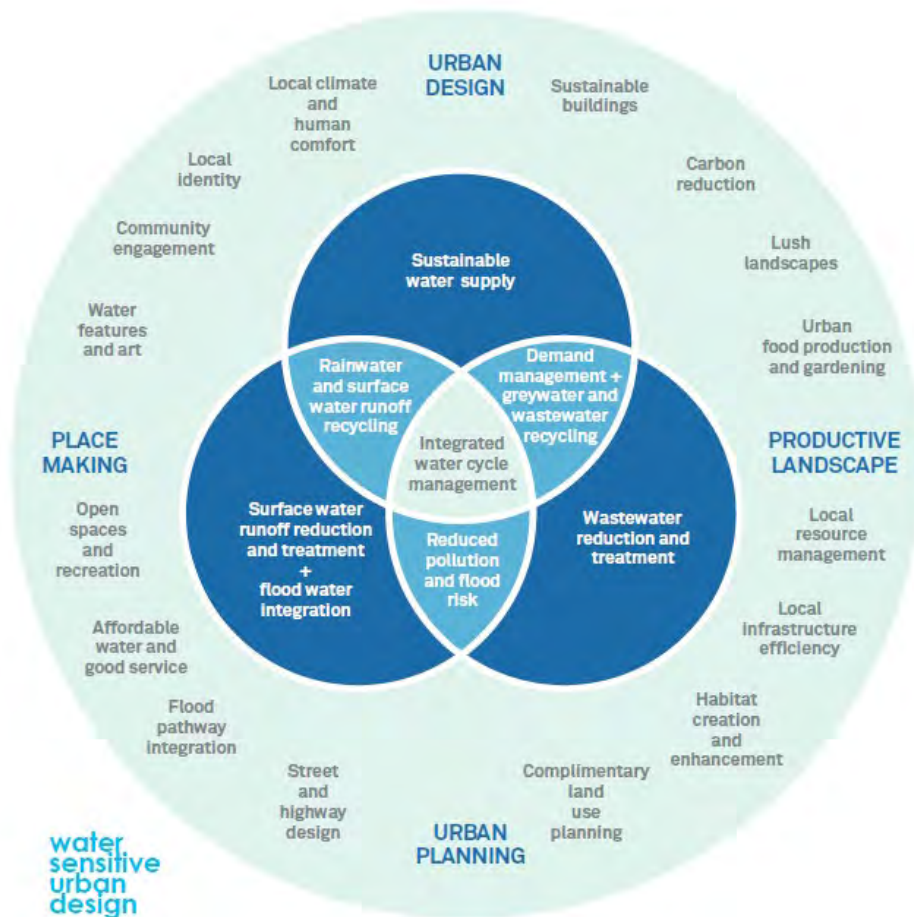
Figure 1: The elements of integrated water management
